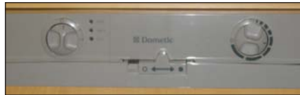
Energy selector switch
